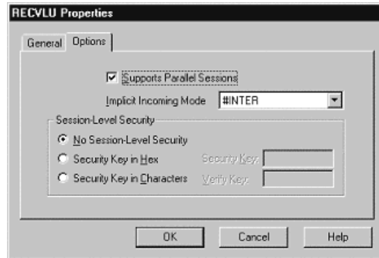
Fig. 223: "MS SNA Server" - Config. of remote APPC LUs (Part 2)
